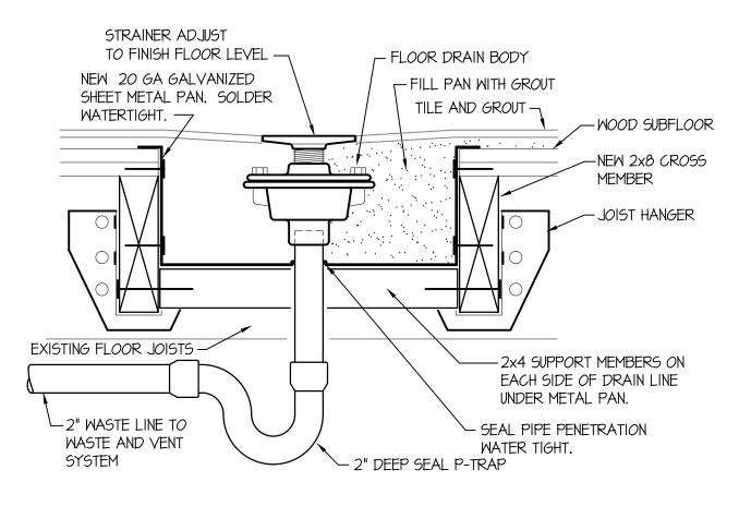
FLOOR DRAIN IN WOOD FLOOR DETAIL NO SCALE
