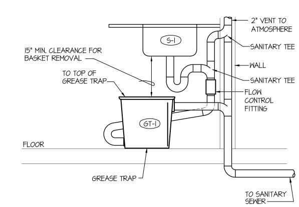
EXPOSED GREASE TRAP DETAIL NO SCALE
